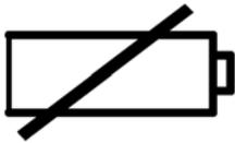
**Low Battery LED:** The low battery LED will flash amber once every second when the onboard 9-Volt battery is near empty. Approximately 20 additional initiate/learn operations can be performed after the battery LED blinks for the first time. The battery LED will light up solid amber during the shut down process to signal that the user can let go of the ON/OFF button.
